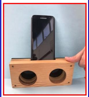
The back of the speakers are made from acrylic, hence the bolts which are visible.
